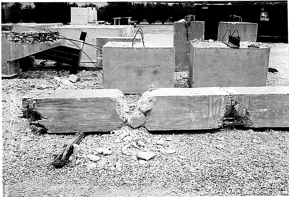
Figure 3.34 Failed Test Specimen Opened for Post-Mortem Investigations
